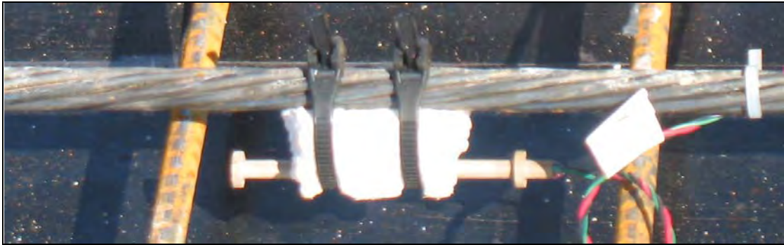
Figure 6.5 Concrete embedment gage installed parallel to a prestressing strand
