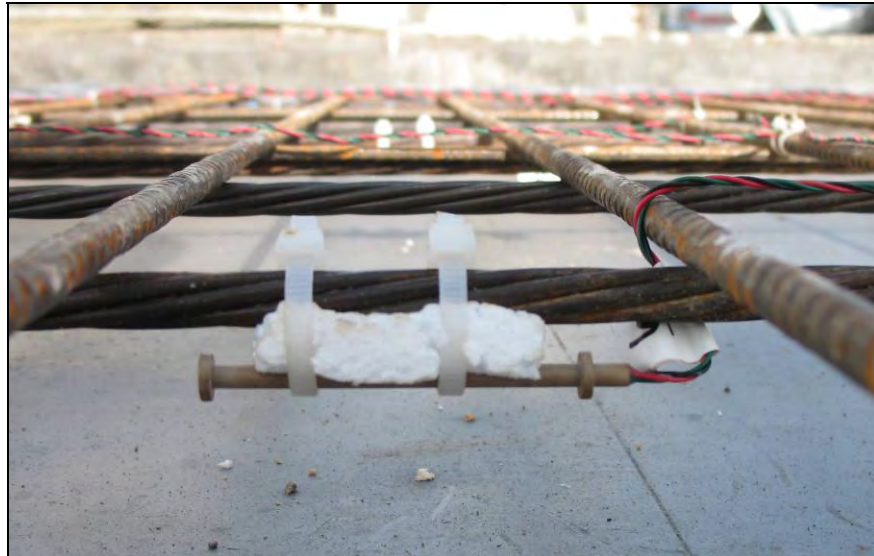
Figure 4.8 Concrete embedment gage installed parallel to a prestressing strand
