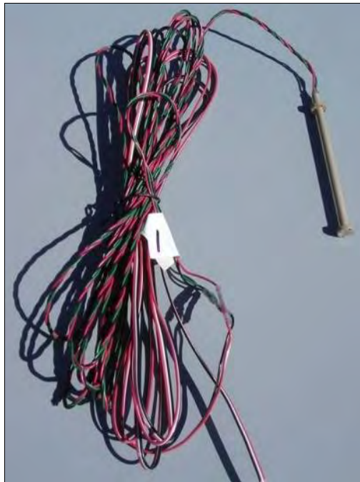
Figure 4.7 Concrete embedment gage (Tokyo Sokki Kenkyujo Co.)
