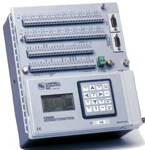
Figure 4.4 Campbell Scientific CR5000 measurement and control system
