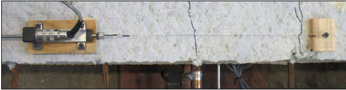
Figure 5.3 Linear potentiometer used with metal wire to measure average strain over center strand
